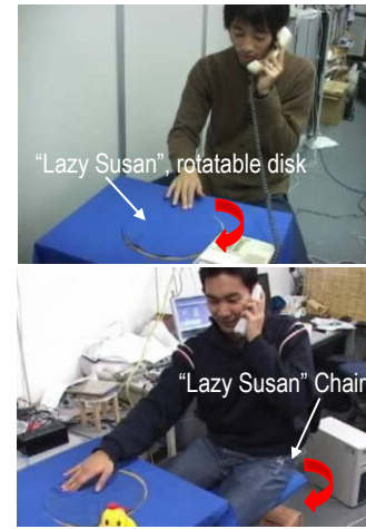
Figure 8: “Lazy Susan” Disk-Chair communication system in use. Rotating your own disk operates a remote chair.
